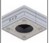
Ceiling installation housing consisting of EPS base body with gluedin OSB rear wall cover and OSB front with cut-out for installation in concrete ceilings.
